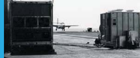
Figure 2. An F-3D Seaknight conducts the first automated landing, aboard USS Antietam, using the radar equipment in the foreground.
