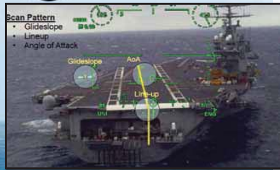
Figure 1. Carrier landing area as seen through the HUD. Pilots need to monitor glideslope using the Fresnel Lens, angle of attack (speed), and lineup simultaneously (background photo: U.S. Navy photo by Petty Officer 3rd Class Kenneth Abbate)
